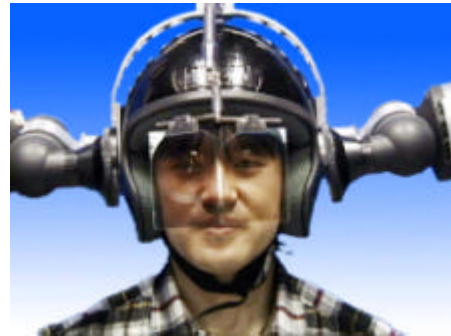
Fig. 12 Head Mounted Projector (HMP) with RPT.
