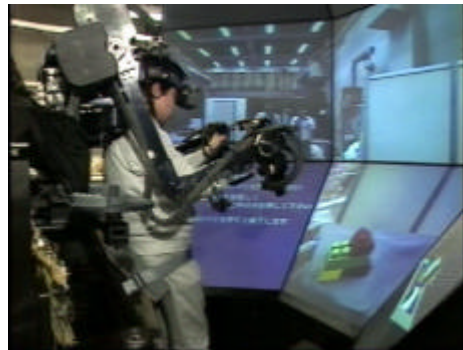
Fig.6 Telexistence Cockpit for Humanoid Control (2000).
