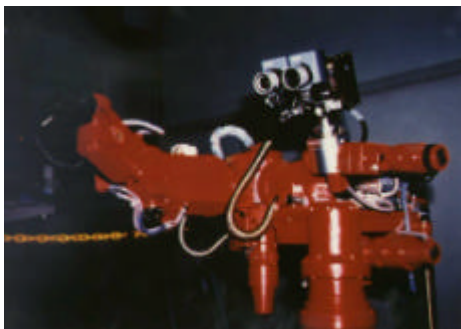
Fig. 2 Telexistence Surrogate Anthropomorphic Robot (TELESAR) at Work (1988).
